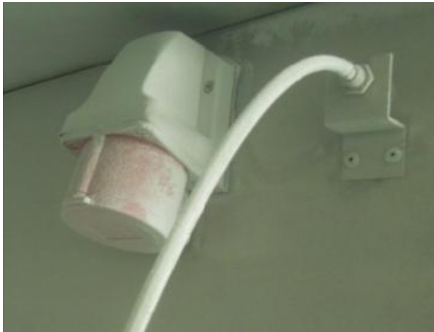
Anti-dust socket for sample connect to power source
