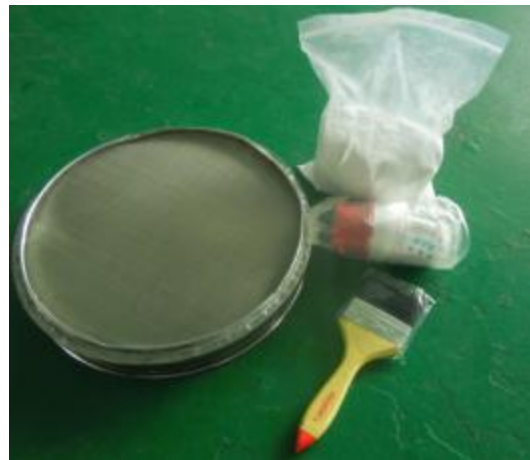
Mesh and parts for filtering test dust
