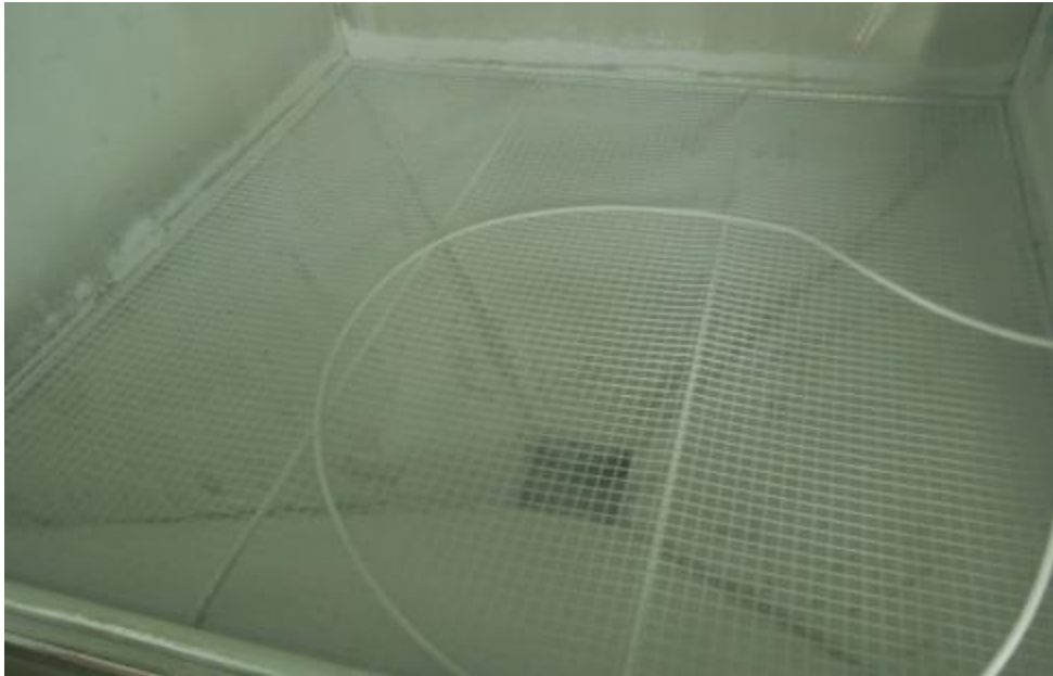
Internal chamber with sample tray & Hopper for dust collection
